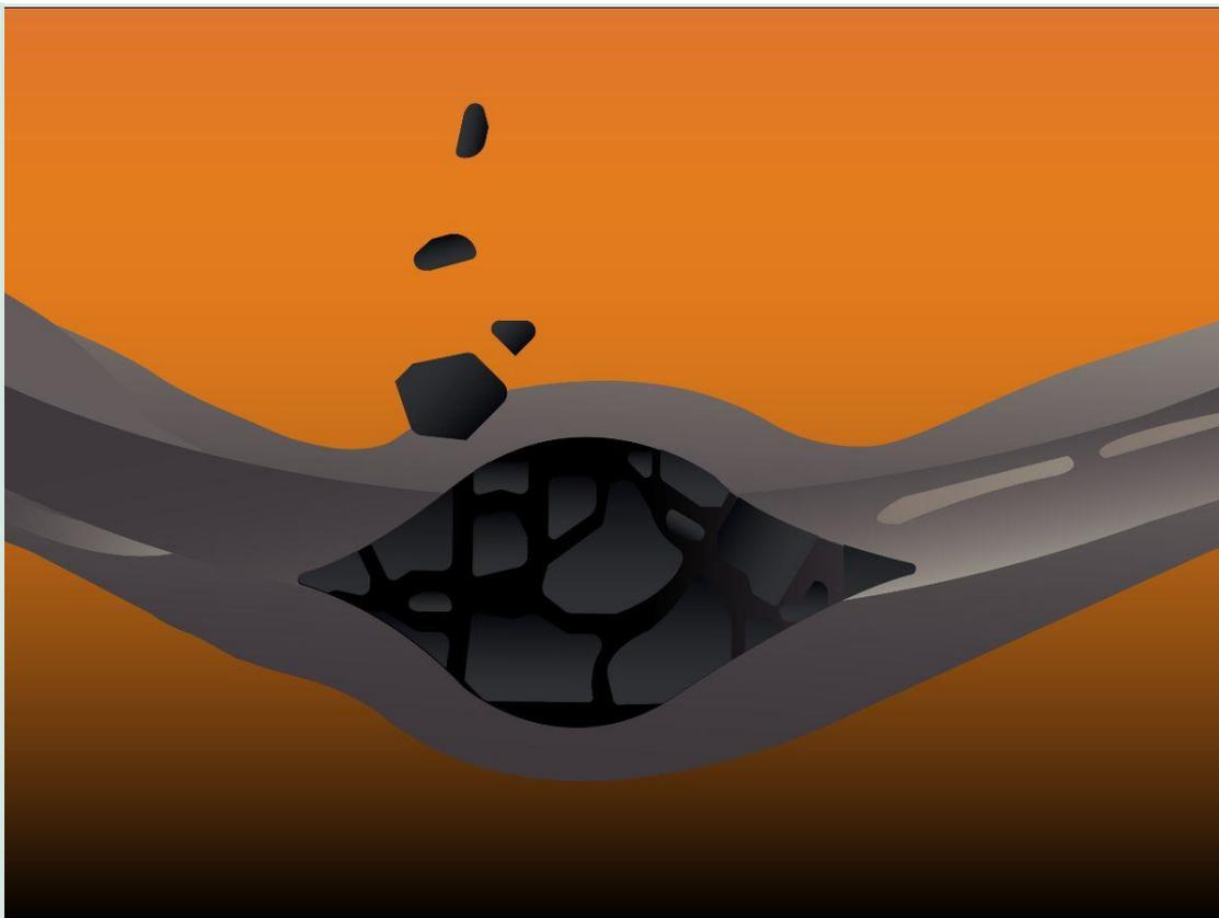
Fuel pellets sometimes degrade to a sandlike consistency and can disperse into the reactor core if a rod’s cladding bursts. ORNL researchers are studying how often this happens and what impact it has, in order to let reactors operate as long as possible without increasing risk. Credit: Jaimee Janiga/ORNL, U.S. Dept. of Energy
