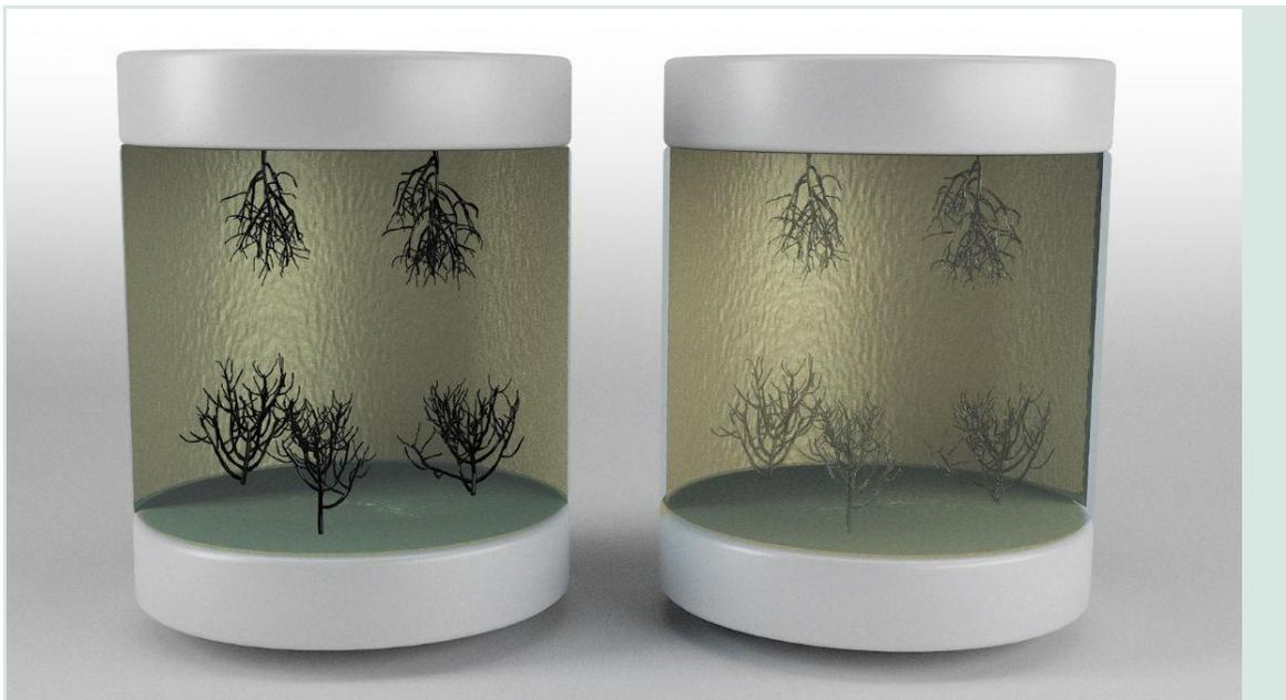
ORNL researchers used an electrochemical process to heal dendrites that formed in a ceramic, garnet-based catalyst designed for a solid-state lithium battery. Credit: Andy Sproles/ORNL, U.S. Dept. of Energy
