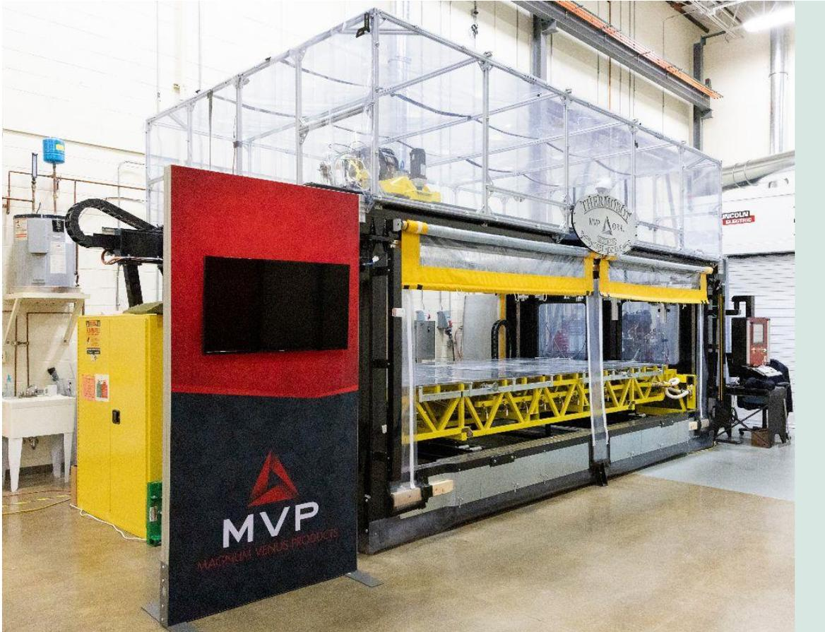
The Reactive Additive Manufacturing Machine was recognized with a 2021 FLC Award. The large thermoset 3D printer was co-developed by ORNL and Magnum Venus Products. Credit: ORNL, U.S. Dept. of Energy
