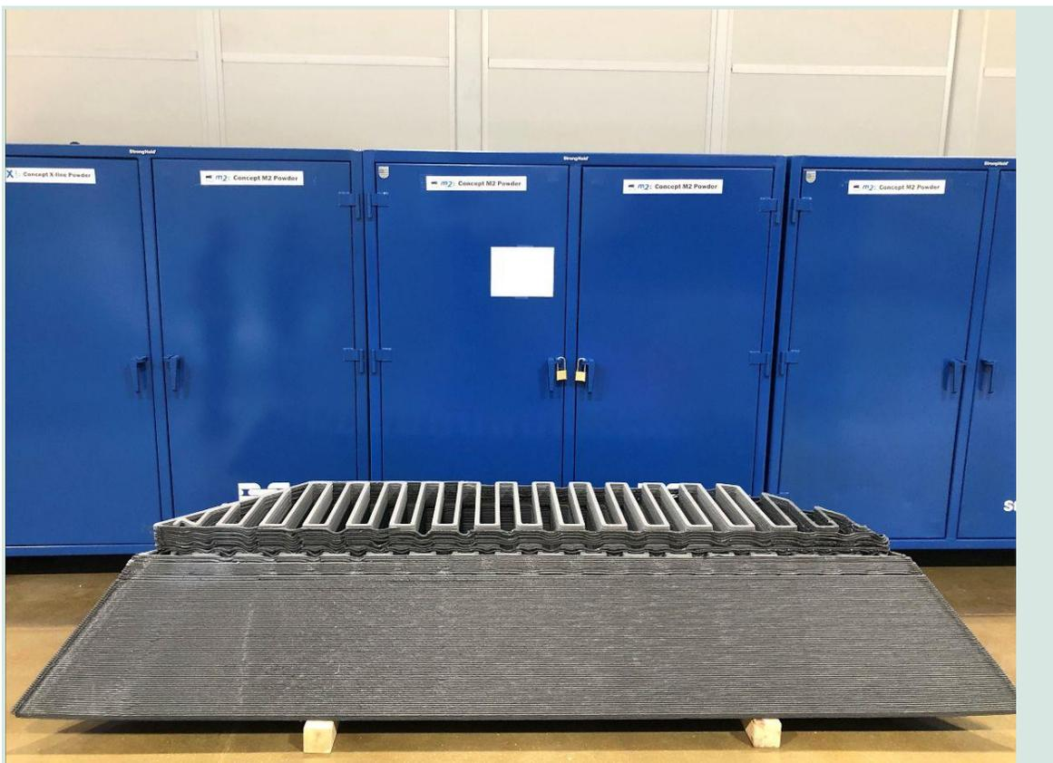
ORNL, in collaboration with Cincinnati Inc., used the Big Area Additive Manufacturing machine to 3D print a mold made of recycled thermoplastic composite and syntactic foam, demonstrating the potential for multimaterials in large-scale applications. Credit: ORNL, U.S. Dept. of Energy
